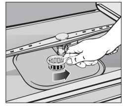
Turn the handle counterclockwise to release the filters.
